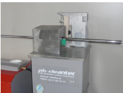
A compact cleaning cell can be integrated into the existing parts handling. Within the cleaning cell spray nozzles are arranged in such a way that the component geometries are rinsed off during circulation.
